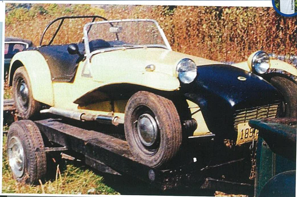
Right: Earliest known photo of 7/B1135, provided by now professional photographer John Heseltine. Note the nearside exhaust of the 1,147cc Triumph engine and the amateurish roll hoop
